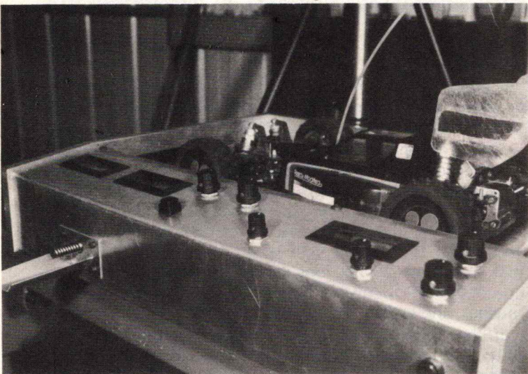
A Dyno. On this machine, motor performance can be tested under load, with the buggy sitting on rollers in the machine. Or, the motor can be tested on its own, by plugging the shaft into the connector on the left of the picture.
